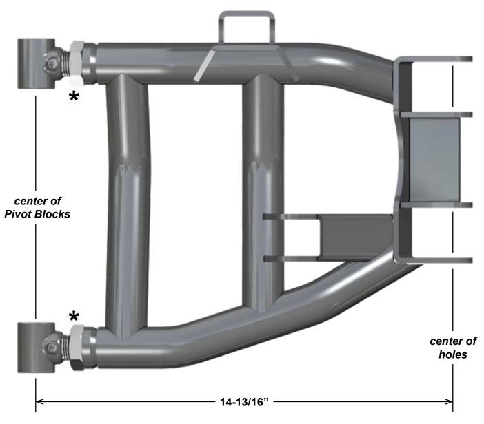
\*Leave Jam Nuts loose. Tighten after final adjustments have been made.
