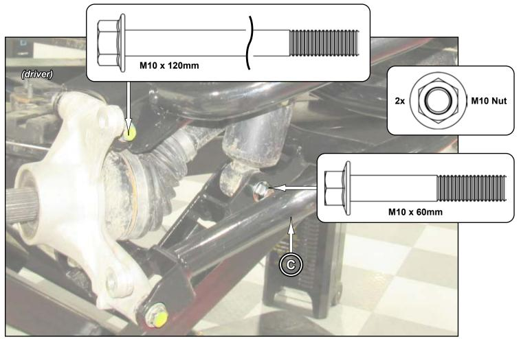
After securing Lower Arms to Knuckle, gaps between Pivot Block faces and Knuckles may be present. Install provided Spacers as shown if applicable.
