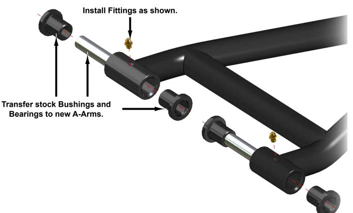
Install A-Arms to Frame and Struts with stock hardware. Tighten completely. SuperATV recommends using Loc-Tite on Nuts when installing A-Arms to Frame.
