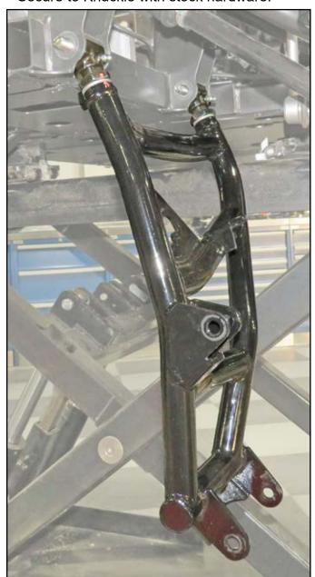
Resecure Swaybar and Shock to Lower with stock hardware.
