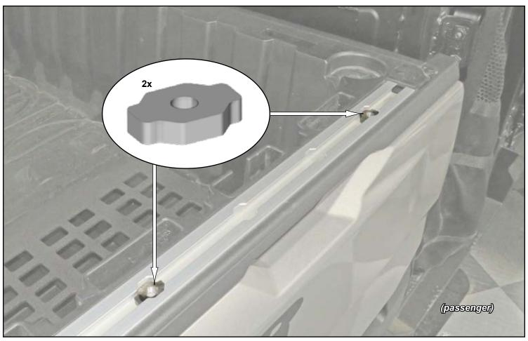
Unless noted, hardware should be snug when installing components; not tight.
