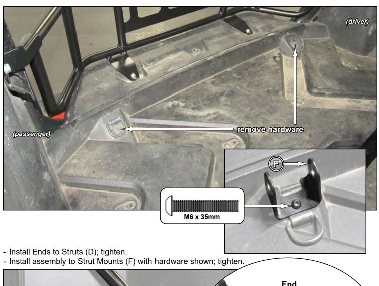
Install assembly to Strut Mounts (F) with hardware shown; tighten.
