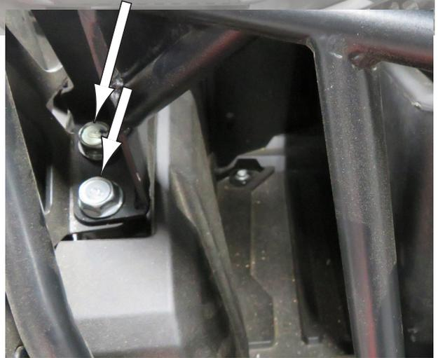
2. Next, install both Left and Right Tube Mount Assemblies (F) and (H), Tube Clamp Brackets (D) using your M6x20 Bolts (C) supplied in your kit. Install but leave a little loose for adjusting fit after all parts are installed. See Fig.2 and Fig.3 for details and basic location where to install them at.
