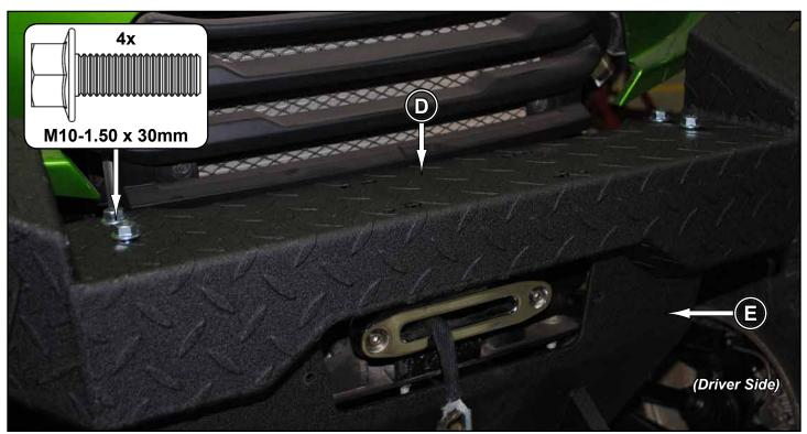
Align to machine and tighten all hardware completely.
