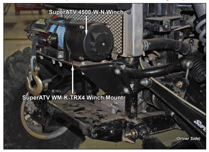
Remove Insert from Lower (D) if a Winch is installed in position shown above.
