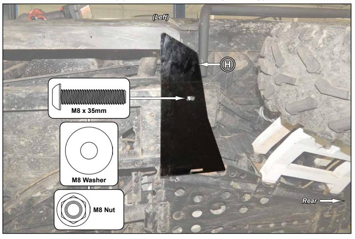
Install Front Plate (A) to Frame with hardware shown.
