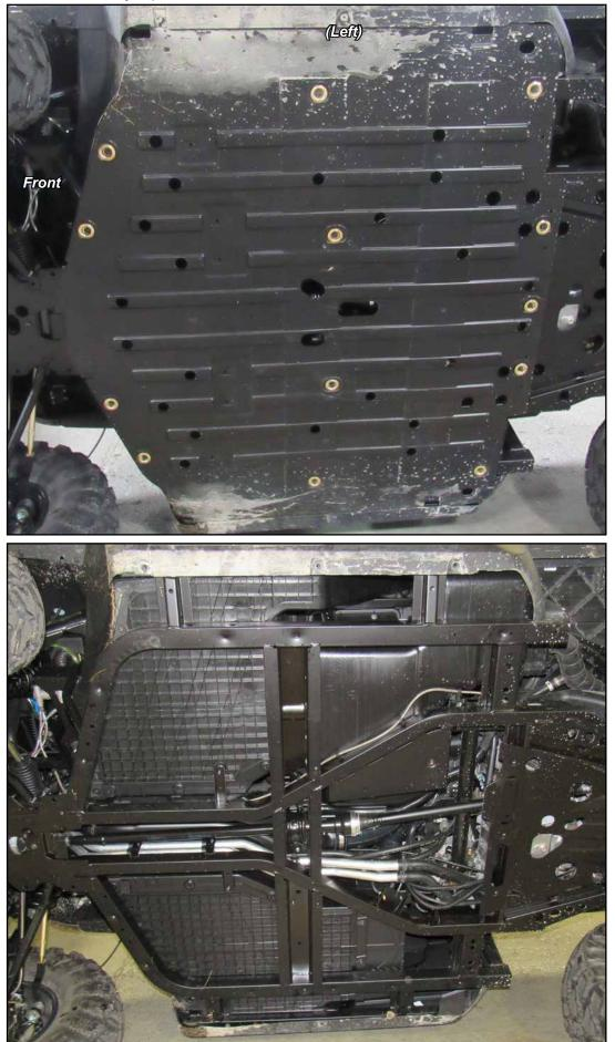
Gently flip machine onto its side and remove stock Skid Plates.
