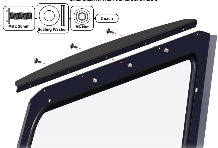
Install Bracket to Frame with hardware shown.
