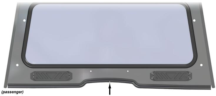
Install Seal to bottom of Frame.
