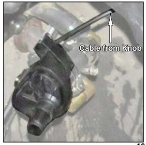
Place Heater assembly into position and location shown.
