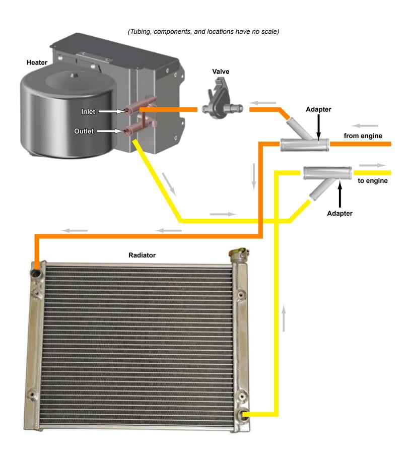
To prevent stock Radiator Hoses from being cut short, use provided Adapters as templates.
