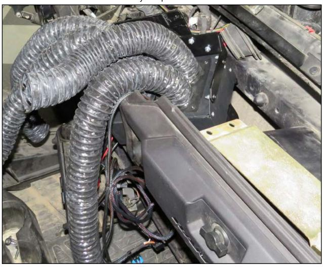
Connect Tubing from Heater to Elbow and Valve with Small Clamps; tighten.
