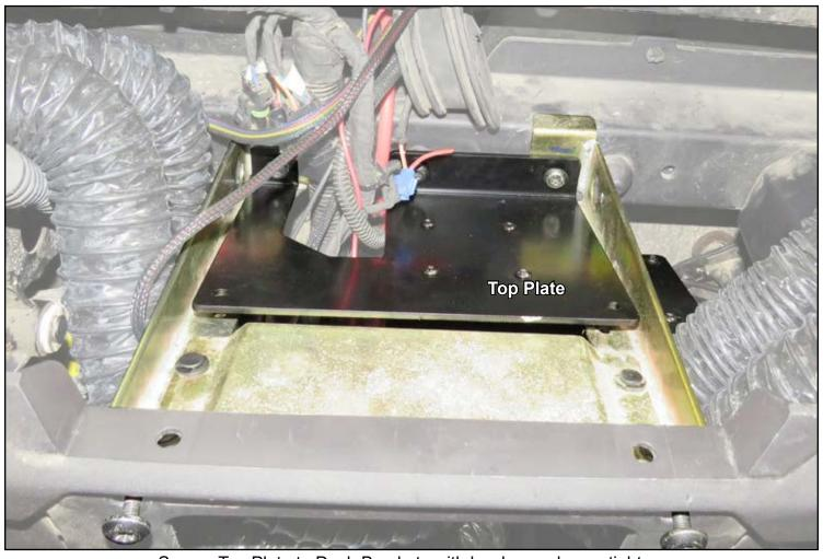
Secure Top Plate to Dash Brackets with hardware shown; tighten.
