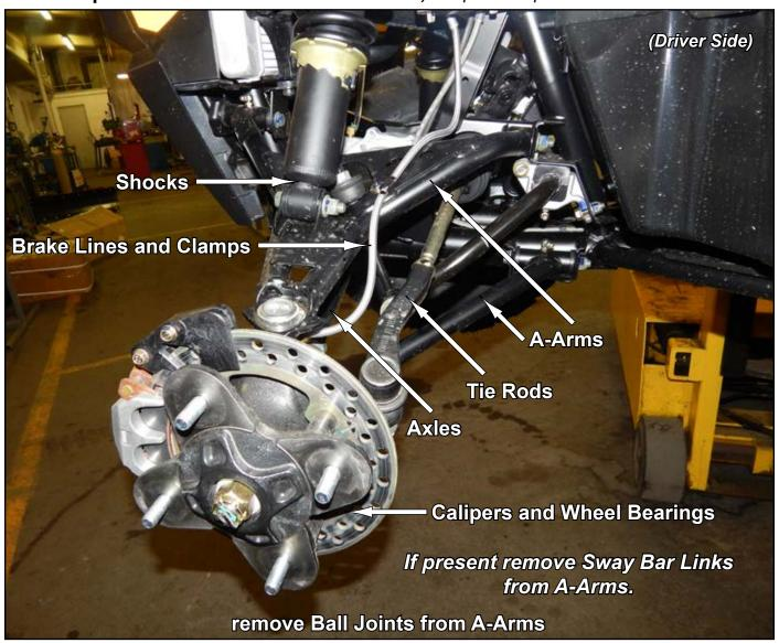
STOCK SWAYBAR AND COMPONENTS WILL NOT BE REINSTALLED.
