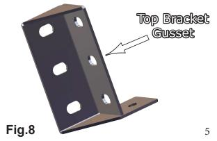
9. Now you need to install the **Top Bracket Gussets** using the **(3) M8x20 Hex Flanged Bolts** and **(3) M8 Nylock Nuts** provided in your kit. Again just snug the bolts as you will need to adjust them later. See **Fig.9**. Repeat for the opposite side.
