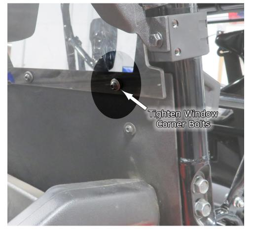
**12**.Now go back and tighten the two (2) back window bolts you loosened up before the installation. Repeat for both sides. See **Fig.12**.
