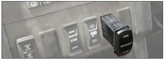
Before permanently mounting Switch, SuperATV recommends testing after all components have been installed. - Secure Switch.
