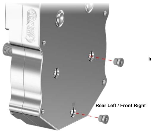
install into each Gear Box Torque to 10 ft/lbs
