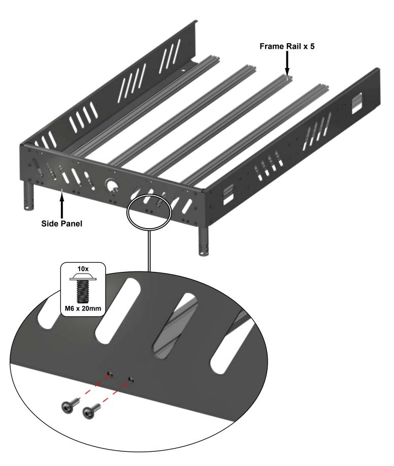
\*If Frame Rails are to be installed to upper position, see page 13 for Hook installation.
