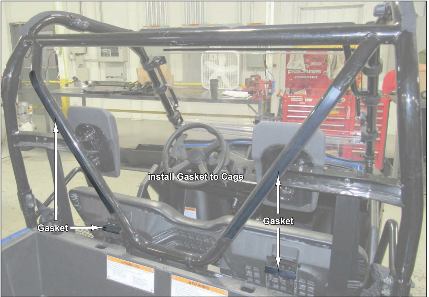
install Gasket to Brackets in location shown
