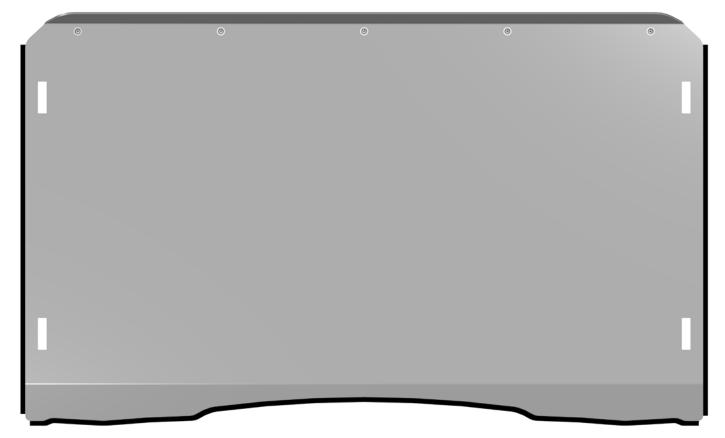
Install Seal along bottom of Windshield.
