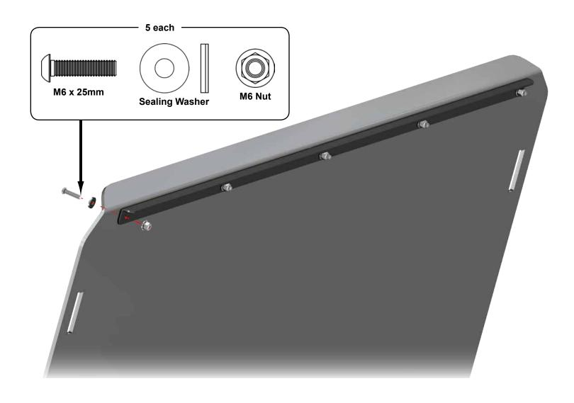
To ease installation, soak Seal and Gasket in hot water before cutting or installing to increase flexibility.
