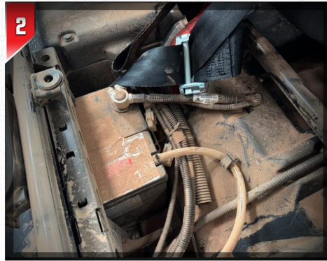
2 Disconnect the battery terminals , starting with the negative (-) cable first.
