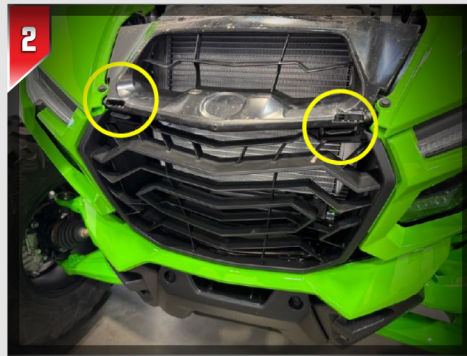
2 Remove the front grille by pressing down on the upper tabs, then pulling it away from the vehicle .
