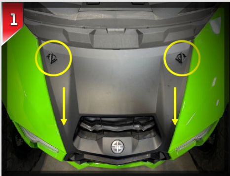
1 Remove the hood by unlocking the two (2) tabs. Lift the hood up and out of the way .
