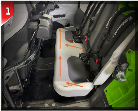
1 Remove the rear seat by pulling up and out .
