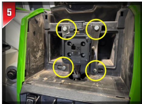
5 Using a Phillips screwdriver and a 10mm socket , remove the four (4) bolts securing the Garmin display mount. Once the bolts are removed, carefully lay the display mount down.
