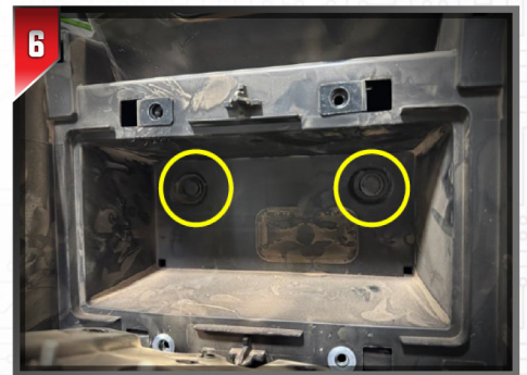
6 Remove the two (2) plastic push pins located behind the display mount.
