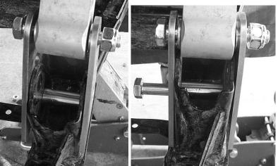
12) Now reinsert the rear spacer between the shock mount tabs and connect it using a 12x80mm bolt and 12mm lock nut.
