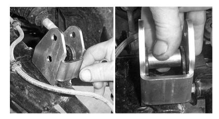
4) Now insert the 10 x 65 hex bolt and secure the bracket and spacer to the frame with the 10mm Locknut.
