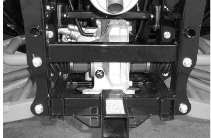
2. Place the logo plate on the frame and mark the hole location for the bracket.
