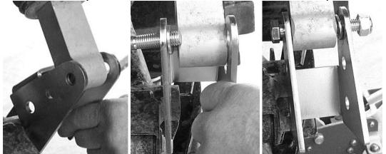
5) Connect the rear lift bracket to the shock mount. Insert the rear spacer between the shock mount tabs where the shock was previously mounted to the shock mount tabs.
