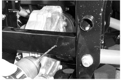
4. Once you have drill the pilot holes, place the logo plate back on the frame and secure it using the two tech screws provided in the kit.
