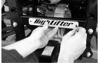
3. Using a small drill bit, drill a pilot hole for the self tapping screws.
