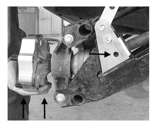
9) Drill the holes on the marked areas. We used the bracket as a guide.
