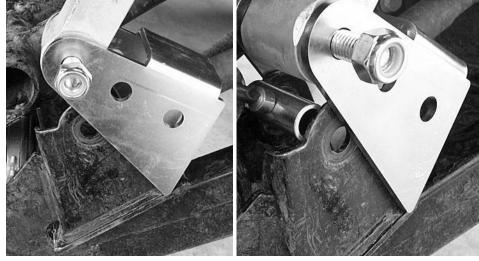
6) <u>Next insert the 12x80mm bolt to hold the spacer and bracket in place and loosely attach the 12mm nut.</u>
