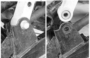
4) Attach the top of the rear lift bracket to the lower shock eyelet using the 12x80mm bolt and 12mm lock nut. Make sure to place a 12mm flat washer on either side of the shock eyelet.
