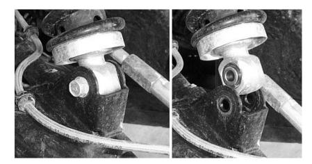
3) Slide bottom of lift bracket over A-arm shock mount and insert one medium spacer between the center of the shock mount tabs and front lift bracket.
