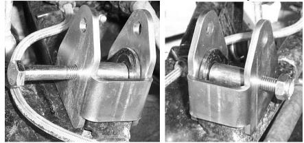
5) Slide bottom of the shock into top of the lift bracket. Using the 10x65mm bolt and 10mm flat washer, insert the 10mm flat washers between the shock eyelet and the bracket. Fasten tight using a 10mm lock nut.
