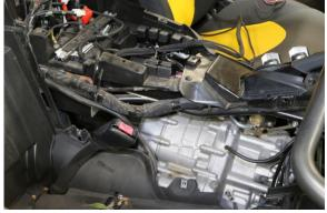
**2.** Mount the control box on top of the center storage box with the  $10-24 \times \frac{1}{2}$ " machine screws provided.
