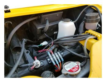
4. Mount Fuse Block. The fuse block can be mounted either inside the glove box or on the outside using machine screws.
