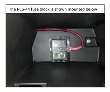
Inside Glove Box - Remove the wires from the fuse block if attached. Mount the Fuse Block inside the rear of the glove box using the #10 self-tapping screws. Drill ¾" hole in the upper left-hand corner of the box, this can be accessed from the front outside under dash cover. Install the provided ¾" grommet, insert fuse block wires into glove box and attach to terminals in the following order; Grey to fuse 1, Orange fuse 2, White fuse 3, Red fuse 4, Blue fuse 5, Green fuse 6, Pink
