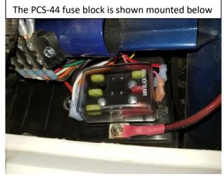
Outside Glove Box - Using the fuse block as a template mark the side of the glove box and drill with  $\frac{1}{4}$ " bit.
