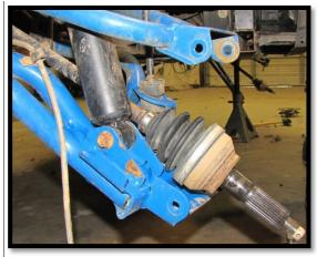
f. While you have the knuckle removed and have more access to the lower arm. You will need to drill/remove the rivet of the p-clamp on the lower factory arm (Or you can simply cut the clamp if you don't want to re-use it). Doing this now will make the new rear brake line installation easier later in the instructions.
