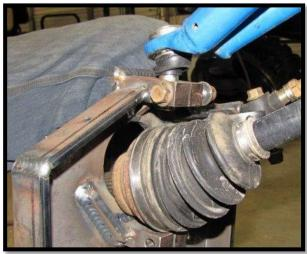
c. Properly position the lower ball joint into the lower ball joint mounting bracket on the backing plate assembly. Then fasten the front lower ball joint with the factory hardware. (15mm)[50 ft lbs]
