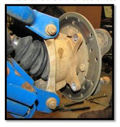
c. Remove the cotter pin and loosen the rear wheel hub castle nut (27mm). Remove the nut from the rear wheel hub assembly. Then remove the brake rotor assembly.
