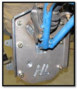
e. Install the tie rod end into the backing plate tie rod mount bracket. Fasten the tie rod end with the factory hardware. (18mm)[90 ft lbs]
