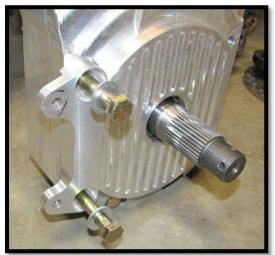
d. Slide a 1/2" flat washer onto (4) 1/2 x 4-1/2" bolts and insert them into the remaining four holes of the box.
