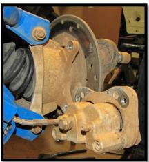
b. Remove the caliper from the rear hub. It is not necessary to remove the brake line from the caliper at this time. Leave the brake hose attached to the caliper and hang the calipers out of the way. Take precautions to ensure the brake hose isn't stretched or pinched.
