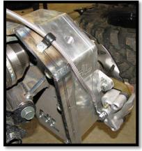
h. Secure the brake lines by using the provided **zip ties**. Make sure there is no binding in the lines once they are secured. (Re-using the factory clamps is optional, but you may need new hardware)
