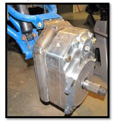
d. Loosely fasten the all four bolts with 1/2" flat washers and 1/2" lock nuts. Recheck all parts that were used and make sure everything fits correctly, and then go ahead and tighten and torque all bolts. (3/4)[105 ft lbs]
