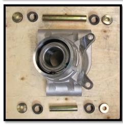
c. Insert the bushings, pivot tubes, and pivot caps into the collars of the **rear right backing plate** (99W-R).
