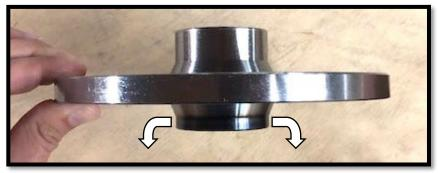
c. With the shorter lip side faced down, find the bolt pattern that corresponds to your make and model. Use the provided studs PGLC-WSTUD-102 (12mm-1.5 stud) (4/156mm bolt pattern)
