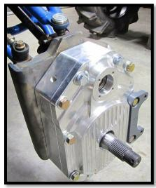
d. Loosely fasten the all six bolts with 1/2" flat washers and 1/2" lock nuts. Recheck all parts that were used and make sure everything fits correctly, and then go ahead and fasten all bolts. (3/4)[105 ft lbs]
