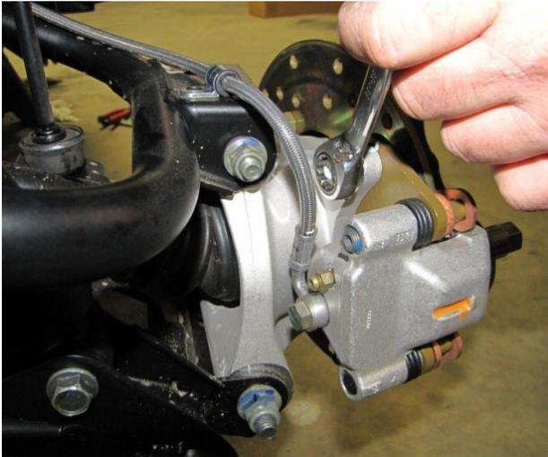
Remove the caliper by removing the (2) stock mounting bolts from the knuckle. (15mm)
