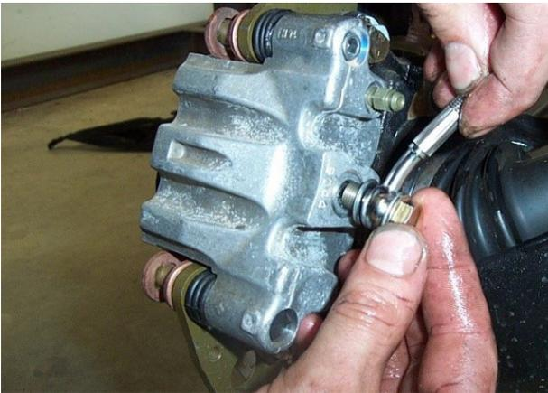
Disconnect the rear factory brake lines from the calipers. Have a container ready to collect brake fluid.
