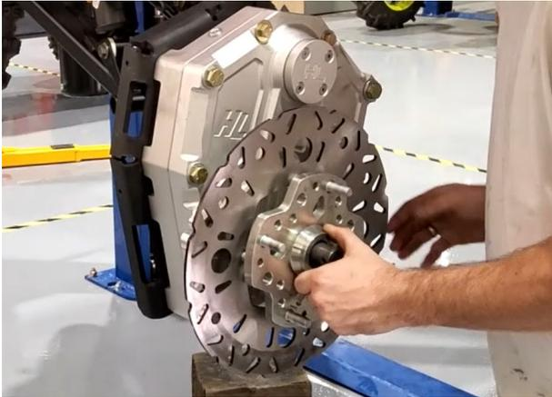
Apply waterproof grease to the spindle splines and slide the brake rotor assembly onto the spindle shaft.
