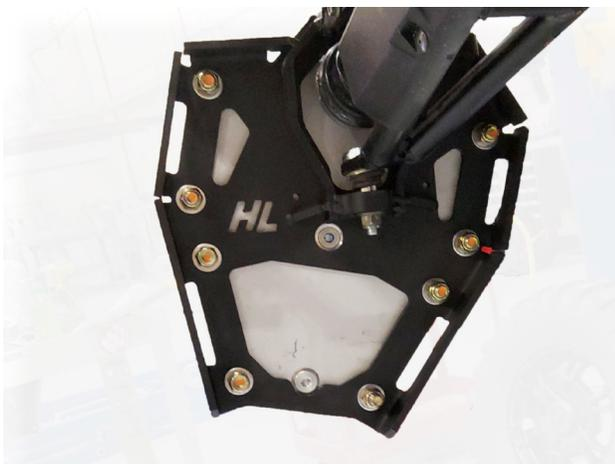
Insert the bolts through the corresponding holes in the backing plate.
