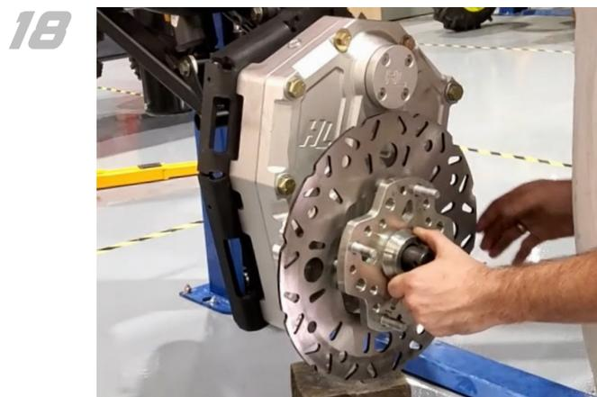
Apply **waterproof grease** to the spindle splines and slide the brake rotor onto the spindle shaft.
