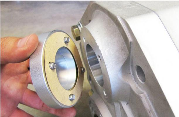
Remove the 1/4-20 x 3/4" screws & cap/gasket from the lid of the **FRONT** portal box.
