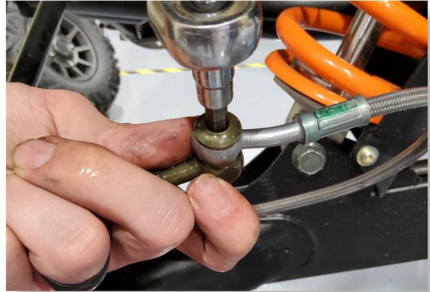
Locate the proper BRAKE LINE EXTENSION. Using the supplied button head hex drive banjo bolt, connect the STOCK BRAKE LINE to the BLIND-END BRAKE LINE EXTENSION. Ensure the copper washers are on each side of the banjo fitting.
