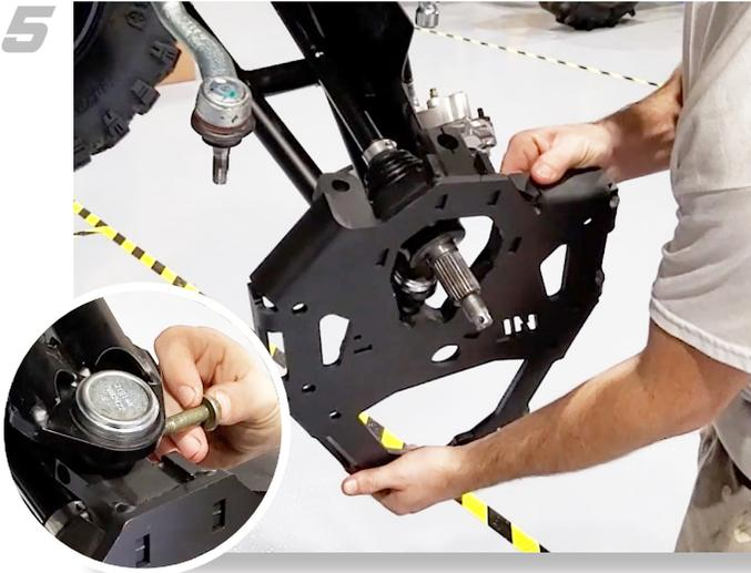
Insert the **lower ball joint** into the lower mount bracket on the backing plate. Loosely secure with factory nut.
