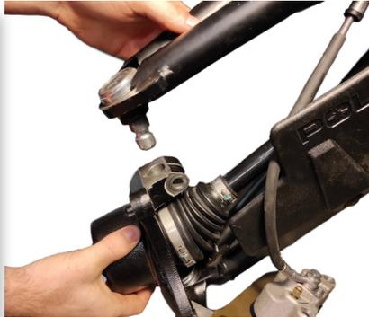
Disconnect the **Upper ball joint** by removing the bolt at the knuckle. (15mm)
