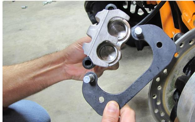
Install the supplied hanger bracket (85X) to the caliper.
