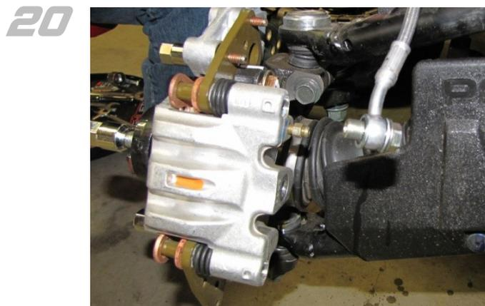
Disconnect the **stock brake line** from the caliper, if you have not done so already. Have a container ready to collect fluid.
