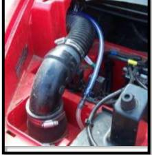
30. Insert the other end into the ½" hole you drilled into the post. Make sure to push the hose up the post as far as you can. Secure the line with (**11**" **zip ties**) provided.
