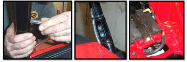
38. On the driver's side of the UTV you will need to drill (2) ½" holes in the cross member on the cage. Drill one lower on the cross member and one higher. The lower hole will be for the rear differential and the higher hole will be for the transmission vent line.
