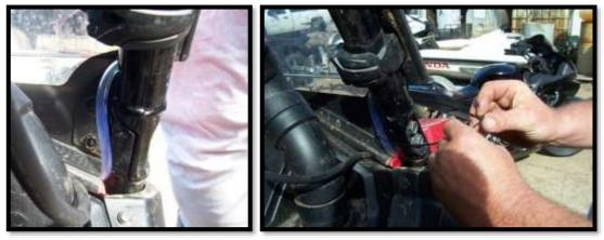
31. The overflow vent line will need to be vented into the cage post on the driver's side of the UTV. It is located on the filler neck of the overflow bottle.
