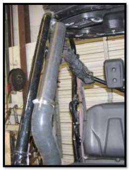
16. Top it off with the riser cap (43R). NOTE: YOU MUST USE SILICONE TO SECURE THE CAP TO THE PIPE
