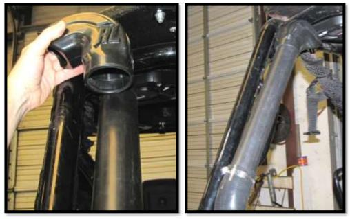
17. Secure the riser to the cage post using (2) of the large wide zip ties (T18HDB).
