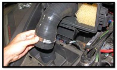
10. Slide the hose onto the intake inlet and tighten the hose clamp. Then slide down and secure the intake box back in place.
