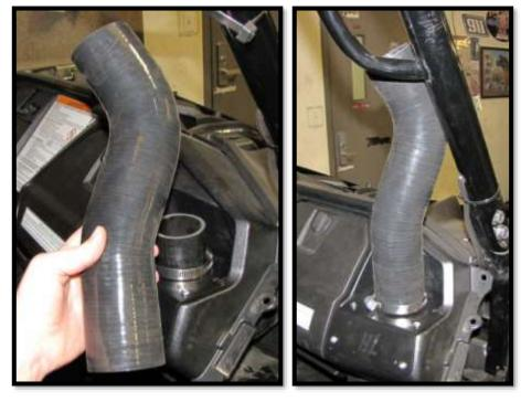
15. Insert the 2" x 16.5" pipe (SK-P-250) into the hose, followed by clamp (HC36).
