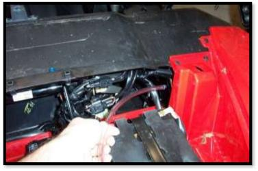
**NOTE:** We removed the driver cup holder so that we could use our fingers to guide the vent line to the location in the plastic where the opening is near the post.
