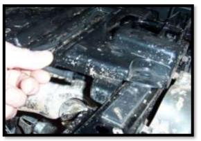
53. Reroute the vent line down closer to the differential. The vent line will have a barb already in it. You need to remove the factory barb.
