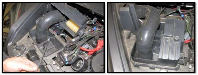
11. At the cup holder, pull the end of the hose out and slide hose clamp (**HC36**) on the end of the hose. Then slide a 2"x3.5" pipe (**SK-P-252**) half way into the hose and tighten the hose clamp.
