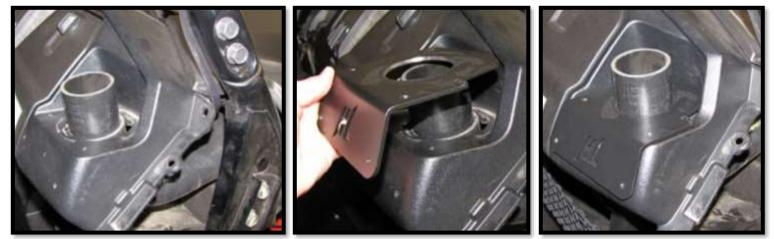
13. Secure the bracket with (5) (PTS1034P) screws. Then slide a hose clamp (HC36) over the pipe.
