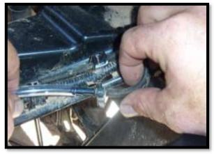
56. Route the rear differential vent line down under the frame or foot rest on the 5 seat version.
