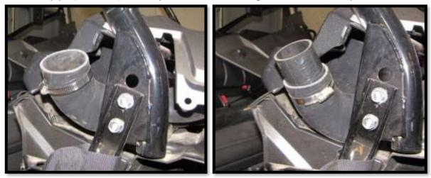
12. Insert the pipe and hose in the cup holder hole. Then slide bracket (80Q) onto the pipe.
