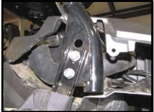
9. Slide the modified plastic cover onto the hose followed by hose clamp (HC52).
