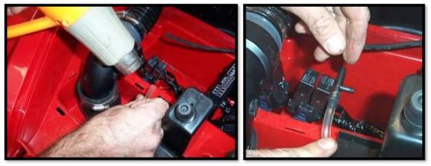
**NOTE:** It will help to heat up the vent line with a heat gun or hair dryer so to make it more pliable so it can fit in the barb.
