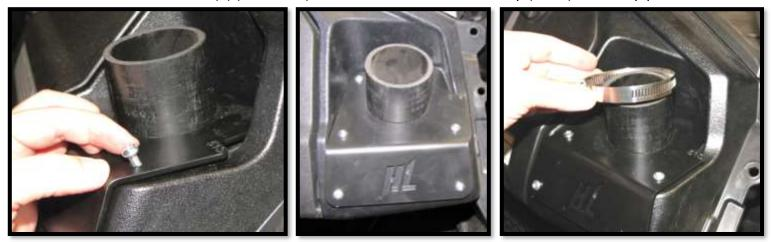
14. Find hose (**78K**). Insert it over the pipe and slide and through the clamp. Then tighten the hose clamp.
