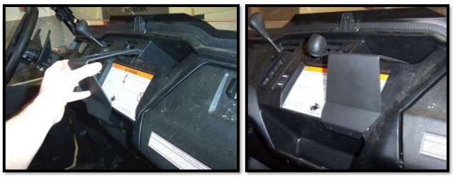
20. Using (4) (**PTS1034P**) screws, attach the bracket to the dash. Then reinstall the factory cup holder into the new bracket.
