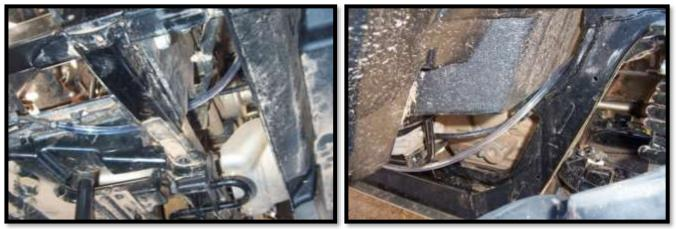
57. Secure the line along the way. Push the vent line up from under the UTV to an opening in the plastic nearest the hole you drilled for the rear differential. Insert the vent line into the hole as far as you can.
