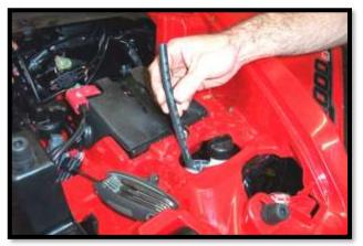
32. Drill a  $\frac{1}{2}$ " hole in the base of the post.
