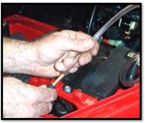
35. Inset the other end of the vent lineup from under the hood through to the hole near the cage post.
