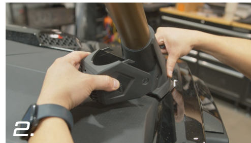
2. Carefully remove the enclosure from the A-Pillar as shown
