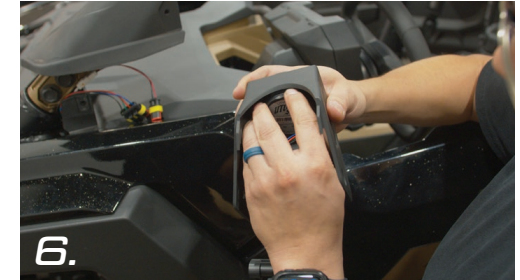
6. Use the locking ring to secure the twitter to the enclosure
