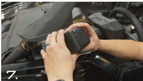
7. Place the OEM grille on to the enclosure
