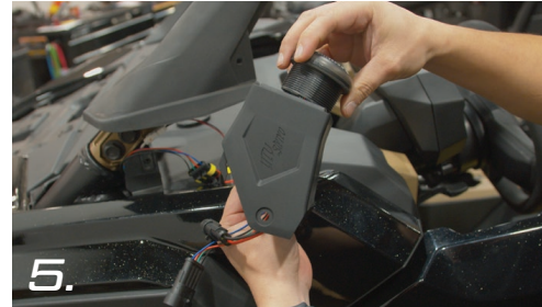
5. Place the tweeter into the UTV Stereo Tweeter Enclosure
