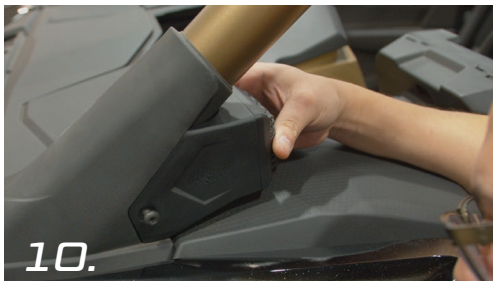
10. Re-attach the OEM hex screws for both sides of the enclosure
