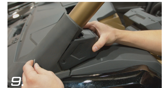
9. Tuck the excess wire into the enclosure and attach the enclosure to A-Pillar
