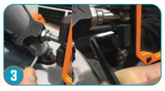
A. Use a 5mm hex key to tighten the clamp into its final position.
