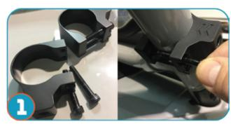
Remove bolts from the supplied clamps and install clamps in the desired position on the cage A-Pillar. Re-install the bolts. Finger tighten.
