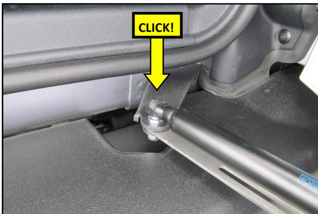
17. Install the OEM gate strut onto the RTR Body Bracket Ball Stud. **NOTE:** The strut body (large diameter) is to be installed on the body side.
