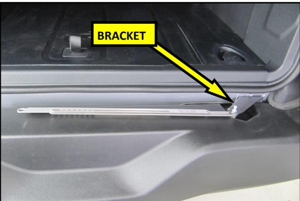
13. Set the Bracket and Link assembly onto the rear bumper as shown, with the Ball Stud pointing upward.
