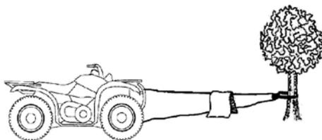
When pulling a heavy load, place a cable hook stopper, blanket or jacket over the cable five or six feet from the hook.
