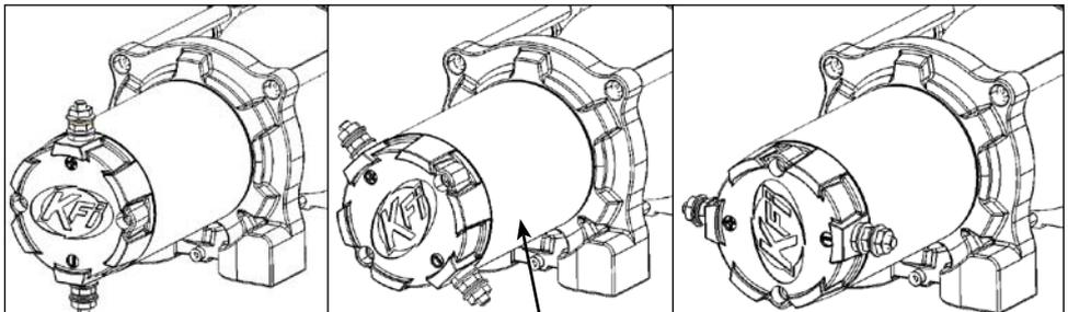
Note: Motor casing rotates with End Cap
