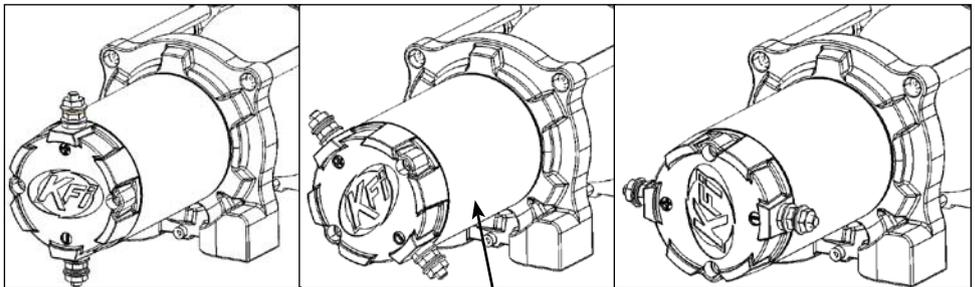
Note: Motor casing rotates with End Cap
