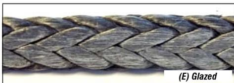
Glossy or glazed sections (see Figure E) in the cable are usually caused by compression, such as the cable being wound on the drum or through a pulley block. This is considered normal.
