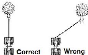
Short pulls from an angle can be used to straighten the vehicle. Long pulls should be done with the cable straight out from the winch/vehicle.
