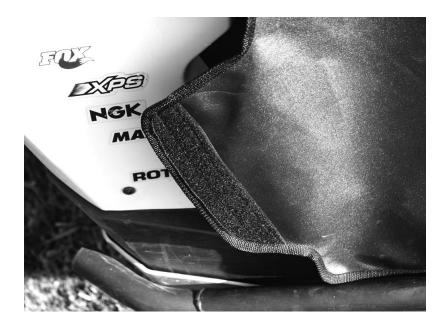
i. Lastly on the door you will take the strap that is sewn to the center webbing strip towards the front of the door and run it through the safety net buckle and back to the ladder lock buckle. You may need to adjust the length so that it is not hard to buckle the webbing when entering the vehicle. See Photo Below:
