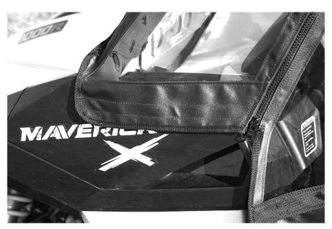
f. The rear of the door has two double-sided Velcro tabs that will attach to the first bar towards the rear of the vehicle. Apply the 6" and 12" adhesive Velcro strips between the horizontal bars facing the rear of the vehicle. (NOTE: You may need to cut the adhesive strips down to fit.) Then attach the double-sided tabs to the adhesive strips as shown in the photo below.
