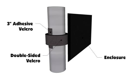
c. Begin installation of the Door Panels by hanging them from the Double-Sided Strips along the top of the doors. Hold the door up and mark where each strip is and wrap a 3" adhesive strip around the roll cage. Now hang the door up and it will be in place to install the rest of the Velcro for the door. See Photo below:
