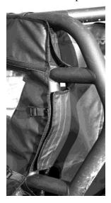
g. Next work your way around the bottom of the door panel and install a snap stud for every snap on the Door Panel. **TIP: You may find it easier to snap the screw stud into the socket on the door first and then pull the Door Panel to the position it should be in and push the screw into the plastic to mark its position. Then remove the screw stud from the socket and drive it into the plastic.** See Photo Below:
