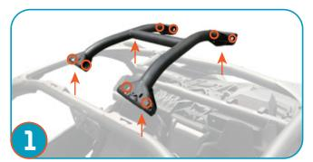
Using a 18mm socket, remove the 8 bolts to remove the stock cross brace.
