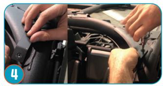
Apply provided bolt tabs to the driver and passenger sides, toward the front of the vehicle, using the provided 2 bolts.
