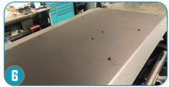
Hand tighten all (8) bolts to allow for adjustment, as needed. Front two bolts will secure bolt tabs (from step 3) and roof to cage.
