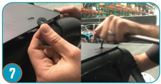
Insert rubber spacers on both driver-side and passenger-side, at rear of roof and tighten bolts securing roof in place.
