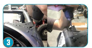
Drill out front and rear driver-side and passenger tabs to allow ease of bolt passthrough.
