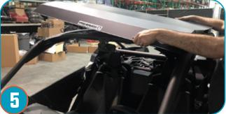
Remove roof from its packaging and place on top of vehicle, ligning up the bolt holes between the roof and cage..
