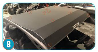
Tighten all bolts (10) to secure roof to cage/vehicle.
