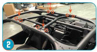
Using an 18mm socket, replace the 8 bolts with provided, Pro Armor cross brace.
