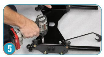
With both seat sliders removed from the car place your new pro armor seat base on and align with the 4 bolts. Re-use the stock bolts that were removed in step 1. Use a 13mm socket.
