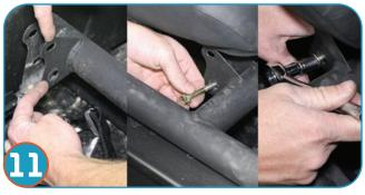
Now align the front of the seat sliders in the bracket and re-use the 2 bolts that were removed in step #3 of the seat base install instructions. Tighten with a 13mm wrench and socket.
