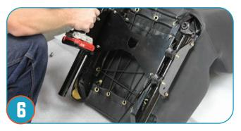
Place your Pro Armor seat face down and attach the seat base to the seat with the 4 ¼-20 bolts that are provided in your hardware pack. Use a 13mm socket or wrench to do this.
