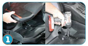
Remove the cushion from the stock seat. Using a 13mm socket, remove the 4 bolts.
