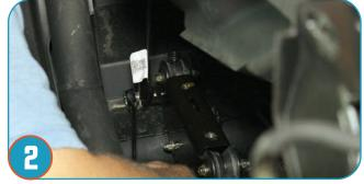
Remove the lower bolt for the stock seat belt with a 16mm socket or wrench.
