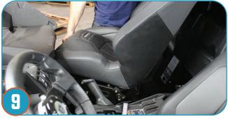
Place the seat in the car and drop the sliders on to the studs so that they are resting on top of the spacers.
