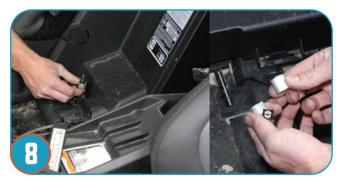
Now you are ready to put the seat back in the car. Place the aluminum spacers on the stud that the seat sliders will be installed.
