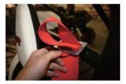
6) Wrap remaining slack up and over buckle, feeding through top slot from the front side and pull tight. Excess slack may be cut or zip tied out of the way. (note: UTV's with many different sized riders will want to keep slack in case of future adjustment). (see photos below)
