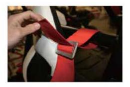
While keeping tension on first wrap feed slack through the bottom front side of buckle, pull tight.(see photos below)
