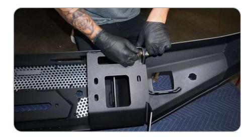
Line up the front and top face of the wings with the center section and tighten all wing hardware using a 21mm socket and wrench.
