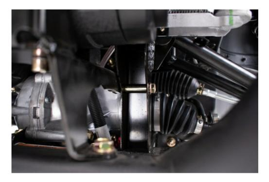
5. Remove the lower mounting points that pass through the bumper structure and thread directly into the frame.
