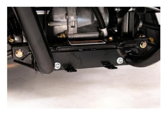
3. Secure the Commander Top Winch Plate to the bumper using the provided **(2) M10-1.5x25 Allen Bolts**, **(4) 3/8" USS Flat Washers**, and **(2) M10-1.5 Nylock Nuts**. Do not tighten.
