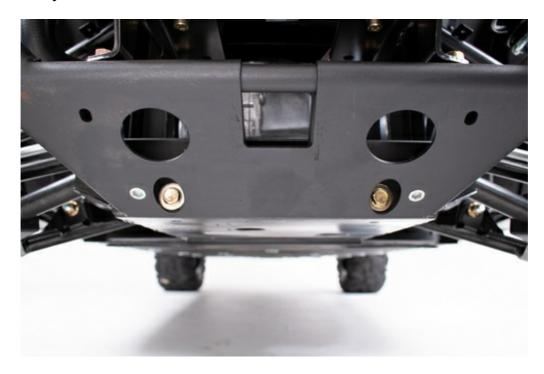
6. Lift and pull forward on the inner bumper to remove it from the vehicle. There are 2 wire hooks built into the bumper holding it onto the frame of the vehicle.
