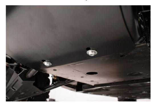
**Note:** If installing a winch and fairlead at this time use the hardware provided with the fairlead to secure the upper mounting points for the skid plate.
