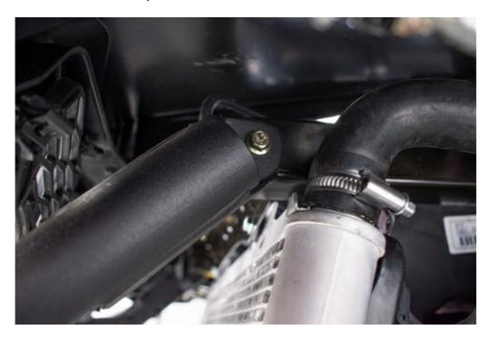
4. Remove the mid mounting points along with the spacers.
