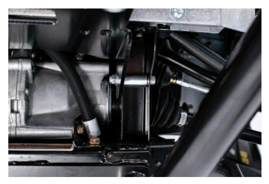
2. Begin installing the front bumper by bringing it up to the vehicle keeping the Commander Top Winch Plate on top of the bumper plate. Use the provided (2) M8-1.25x25 Allen Bolts and (2) 1/4" Flat Washers to secure the lower mount. Do not tighten.
