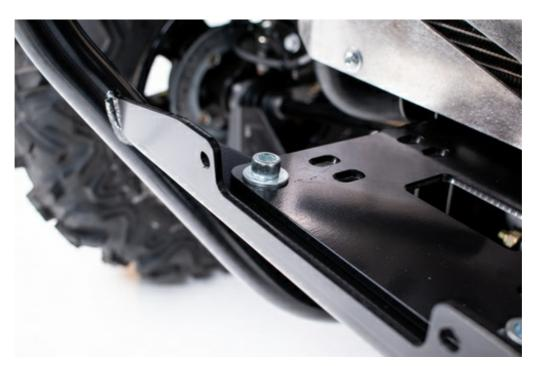
4. Position the **Commander Support Arms** as shown with the arm under the mounting hole in the light bar plate and going up to the upper mounting point on the frame. Loosely secure the support arm to the bumper with the provided **(2) M8-1.25x20 Buttonhead Bolts, (2) M8-1.25 Nylock Nuts, and (4) 1/4" Flat Washers.**
