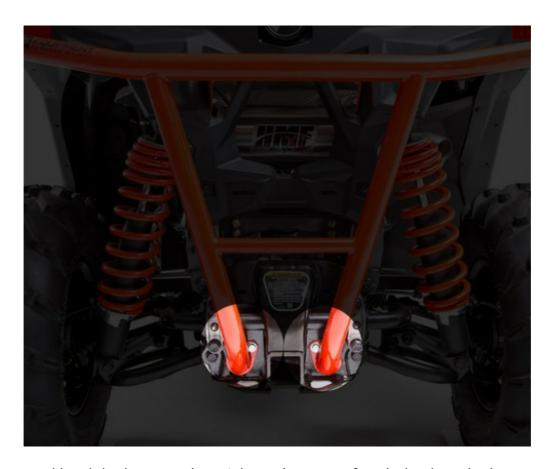
4. Center and level the bumper then tighten the upper four bolts then the lower two.
