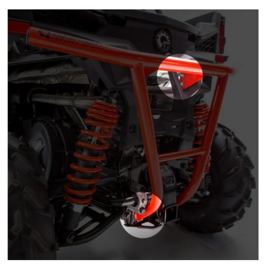
3. Install the (2) M8x25 Hex Bolts, (4) 1/4" washers and (2) nylocs to the lower portion of the vehicle's frame.
