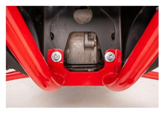
10. Secure the winch plate to the previously installed Mid Plate using the provided (2) M8-1.25x20 Hex Bolts, (2) M8-1.25 Nylock Nuts, and (4) 1/4" Flat Washers.
