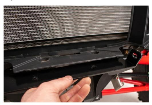
5. Secure the grill surround to the mid plate at the center holes and corresponding holes in the grill surround using the provided (2) M6-1.0x16 Flanged Bolts, (2) #10 Flat Washers, and (2) M6-1.0 Nylock Nuts.
