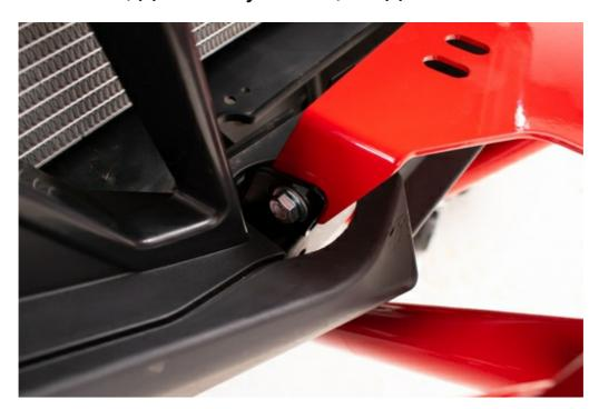
11. Secure the main bumper top tube to the previously installed Side Brackets using the provided (2) M10-1.5x25 Allen Bolts and (2) 3/8" USS Flat Washers.
