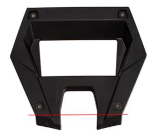
4. Install the provided **U4 Front Bumper Mid Plate** using the provided **(2) M8-1.25x20 Hex Bolts, (2) M8-1.25 Nylock Nuts, and (4) 1/4" Flat Washers** where the origal front bumper hoop mounted.
