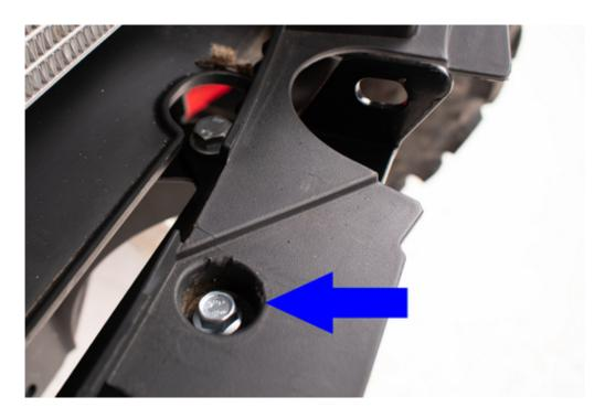
6. Temporarily remove the 10mm head flanged head bolts for the fascia supports and place the provided **U4 Front Bumper Side Brackets** between the support and frame of the vehicle. Secure the brackets using the provided **(2) M10-1.5x25 Allen Bolts**, **(4) 3/8" USS Flat Washers**, and **(2) M10-1.5 Nylock Nuts**. Reinstall the original bolts for the fascia support.
