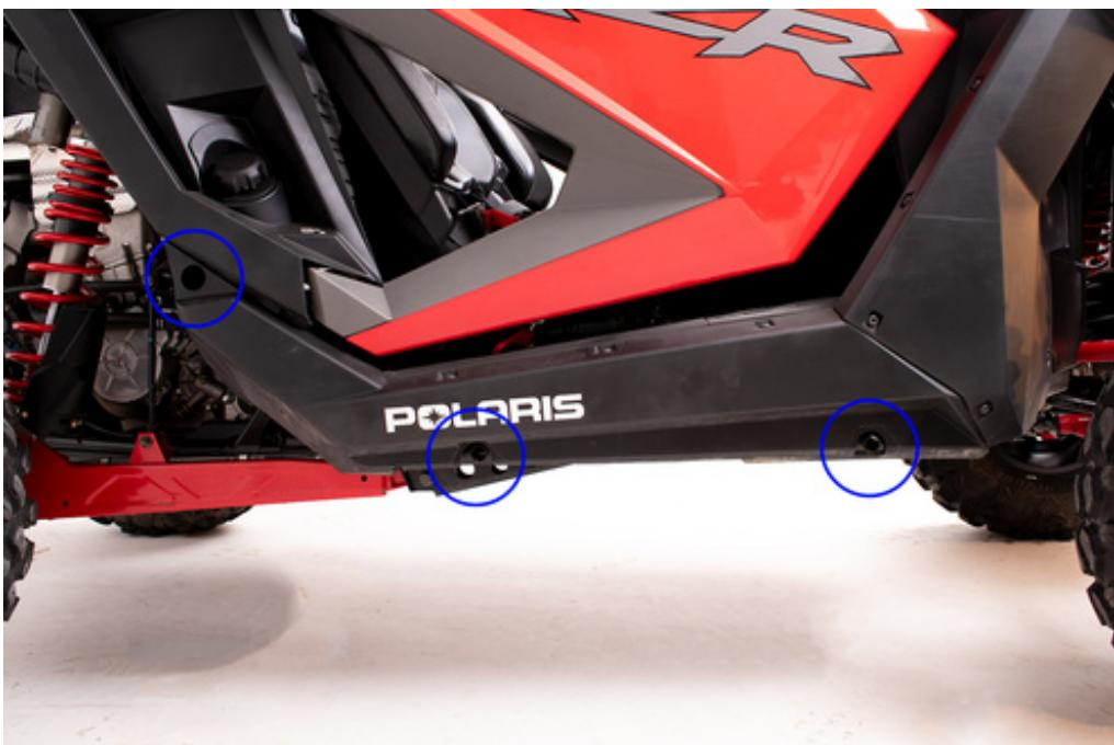
3. Slide the provided **Rock Slider Aluminum Spacers** into the (3) mounting locations on each side of the vehicle.
