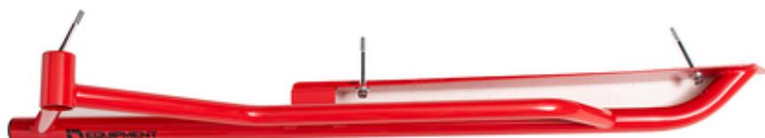
5. Lift the rock sliders into place and slide the bolts through the previously installed spacers. Secure using the provided **3/8" Fender Washers, and M10-1.5 Nylock Nuts**. Do not overtighten the mounting hardware.
