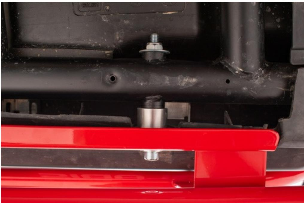
**Note:** The forward mounting points are accessed from under the vehicle, the rear mounting point is accessed by reaching behind the seats.
