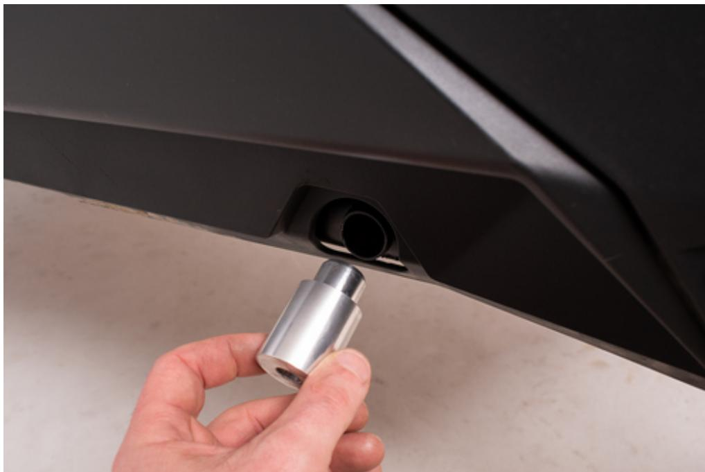
**Note:** Make sure the bungs in the vehicle's frame are clean, if any debris is left in the bungs the provided aluminum spacers will not seat properly. Additionally, weld splatter from the manufacturing of the vehicle may still be present inside the bungs. If this is the case the spatter will have to be ground out in order for the spacer to fit properly.
