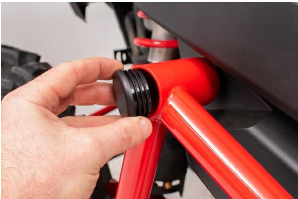
7. Reinstall the skid plate if completely removed. Ensure that the rock sliders go over and below the outer edge of the skid plate. If the skid plate is not tucked above the mounting plate for the rock sliders it will not reinstall properly.
