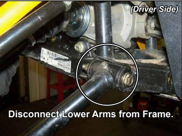
Do not tighten hardware completely unless noted.
