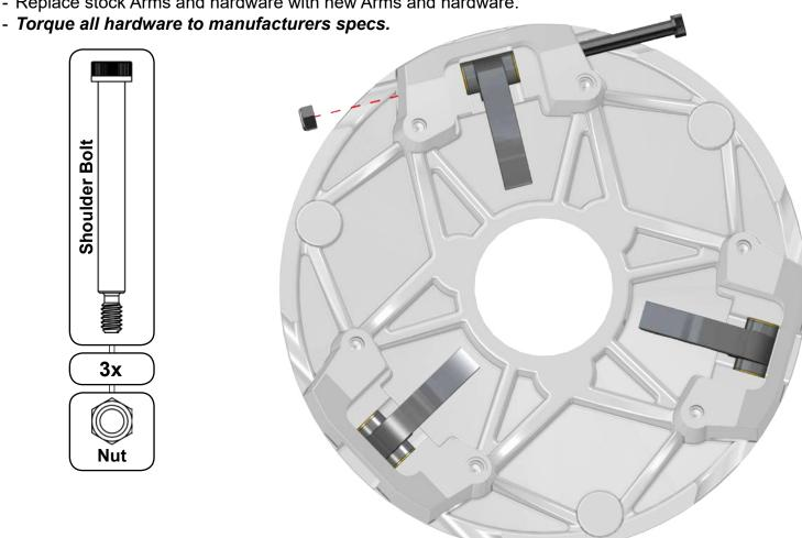
More Heel Weight: lowers engagement RPM and machine will pull stronger on take off (big tires). More Tip Weight: lowers shift RPM but will make upshifts harder. Shift point RPM is also lower.
