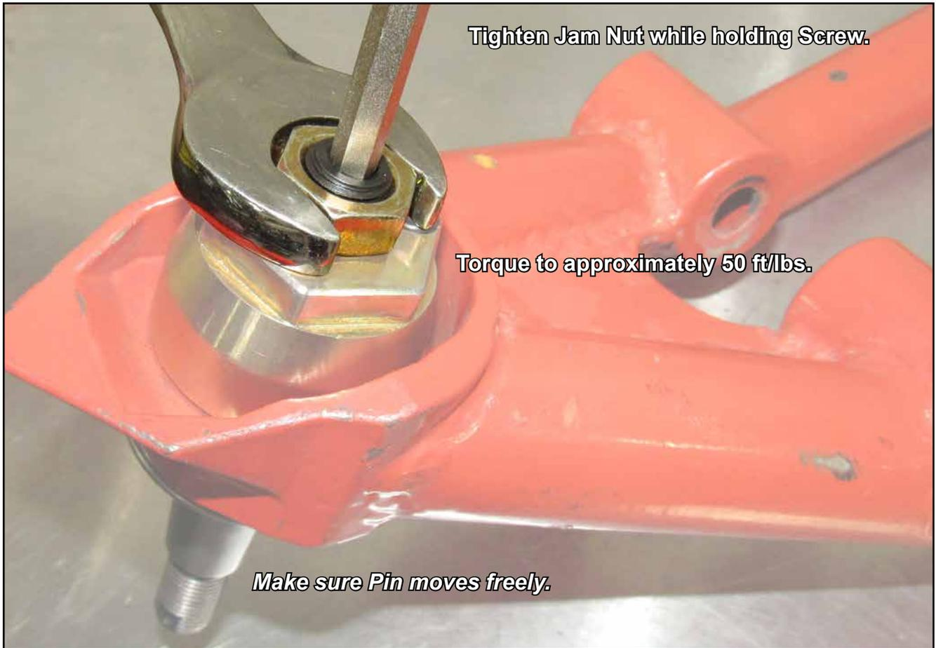
**Tighten Jam Nut while holding Screw.**
