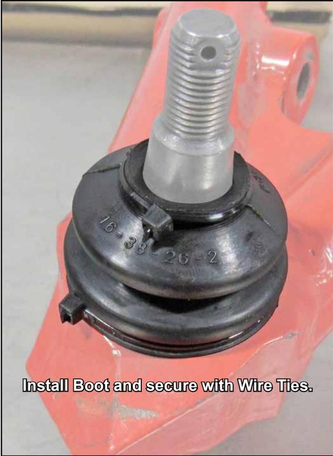
**Install Boot and secure with Wire Ties.**
