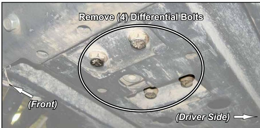
**Bolts should thread easily into Differential. If resistance occurs, stop and use other bolts included with kit.**
