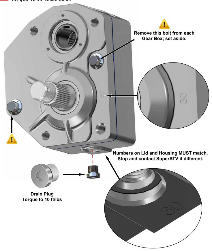
DO NOT USE IMPACT WRENCH WHEN INSTALLING ANY HARDWARE INTO HOUSING
