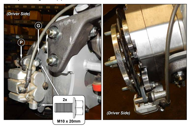
Tighten hardware completely and repeat steps for opposite Brake Caliper.
