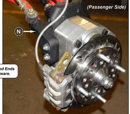
Rear: do not tighten hardware completely unless noted.
