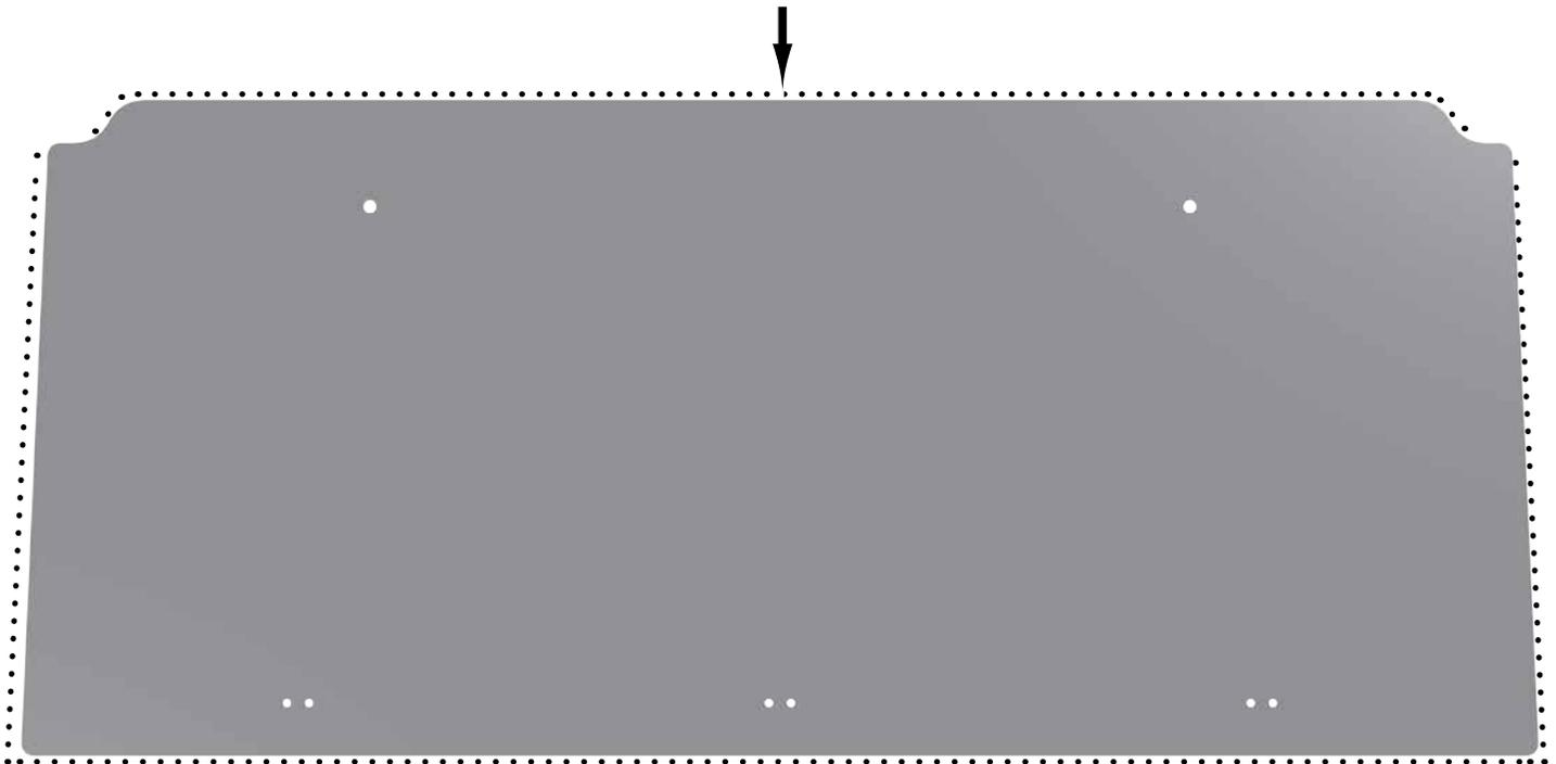
**install (1) piece of Seal to sides and bottom of Windshield (A)**
