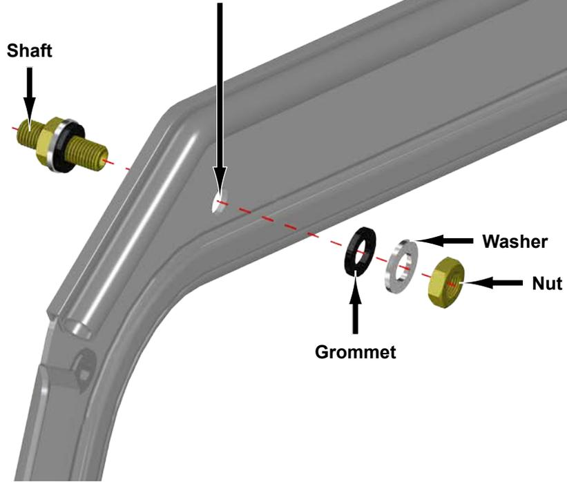
**install Wiper and Handle; do not tighten completely**
