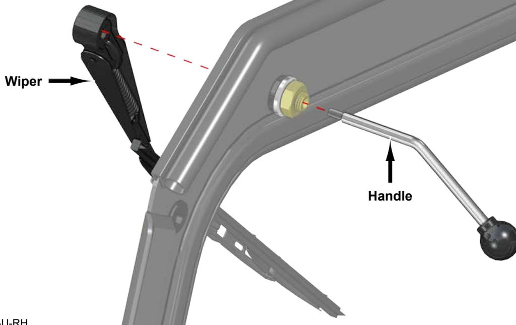
SuperATV recommends positioning Handle and Wiper as shown; tighten completely
