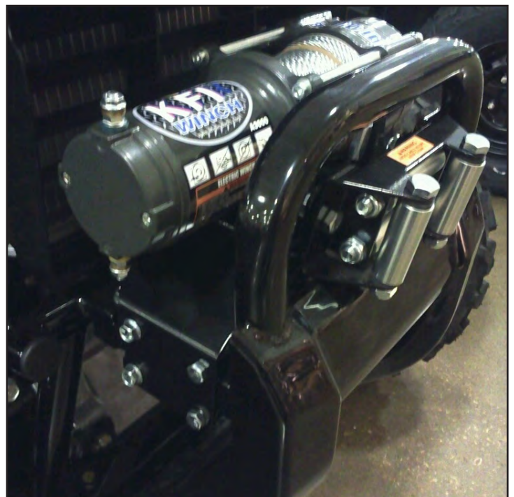
“Figure 8 Winch and Mount Installed”
