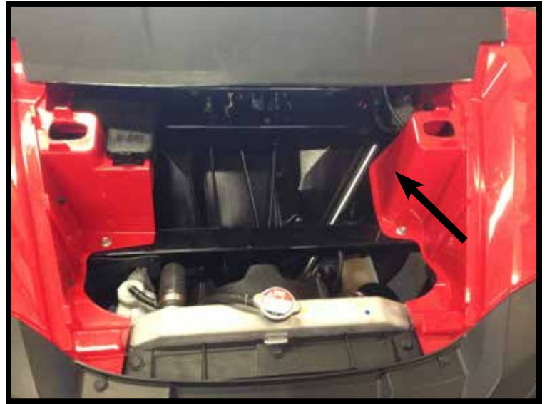
“Figure 7” Contactor Location
