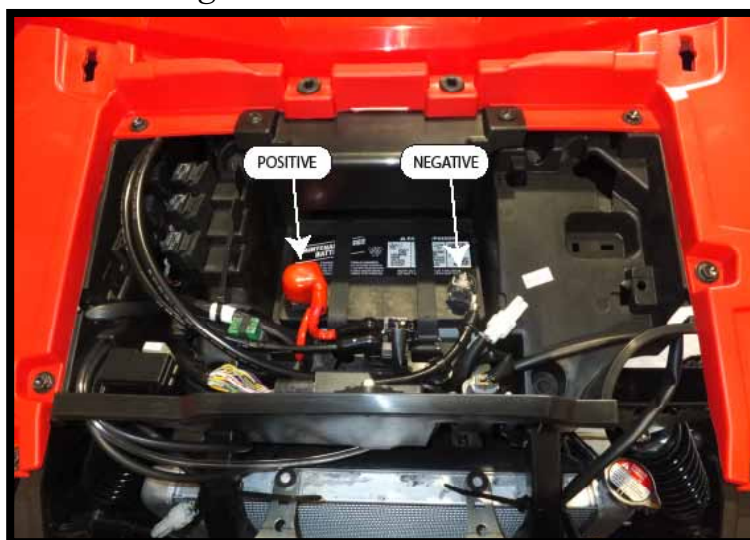
“Figure 9” Battery Location
