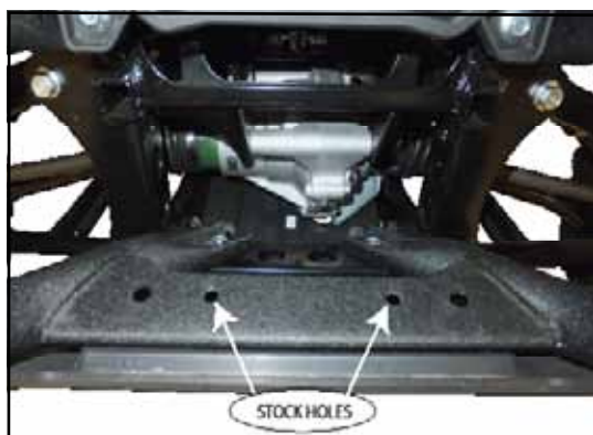
“Figure 5” OEM Bumper Bracket
