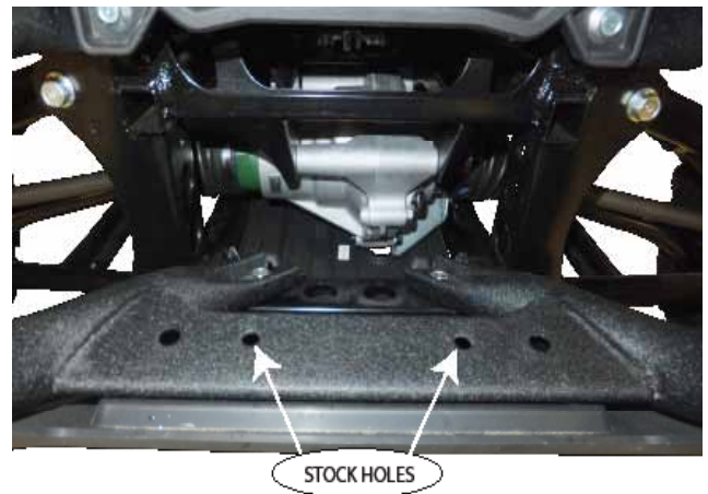
“Figure 7” OEM Bumper Bracket
