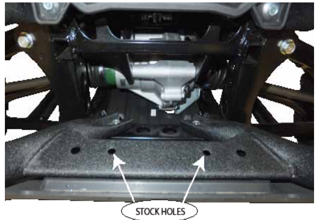
“Figure 10” OEM Bumper Bracket
