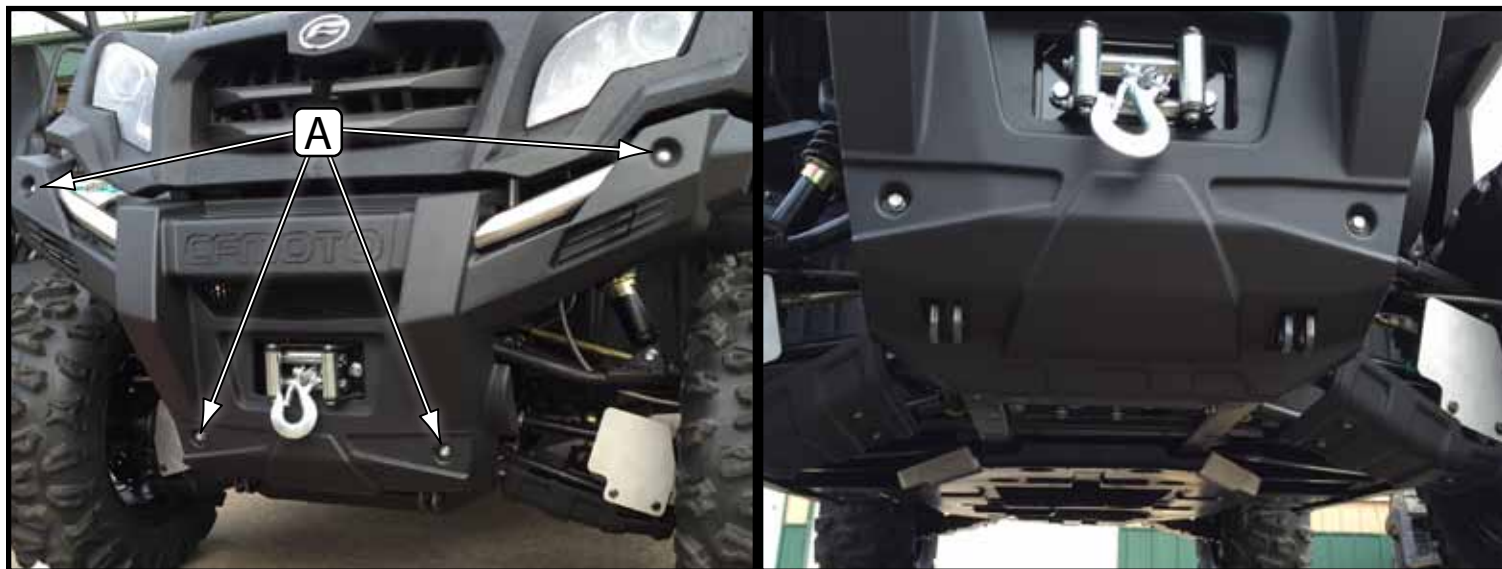
“Figure 6” Plastic Re-Install
