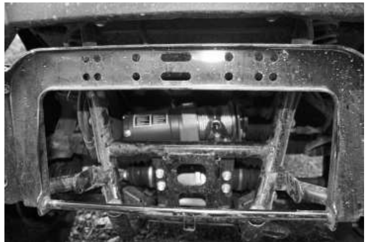
Figure 2 Place Winch Inside The UTV Frame
