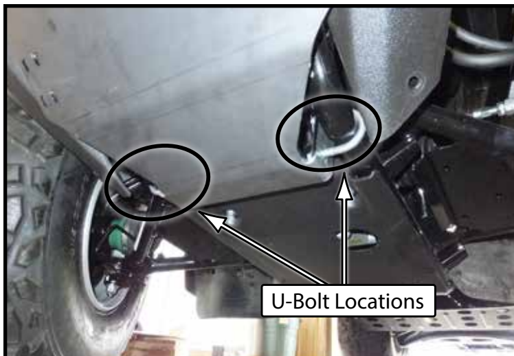
"Figure 3" U-Bolt Install
